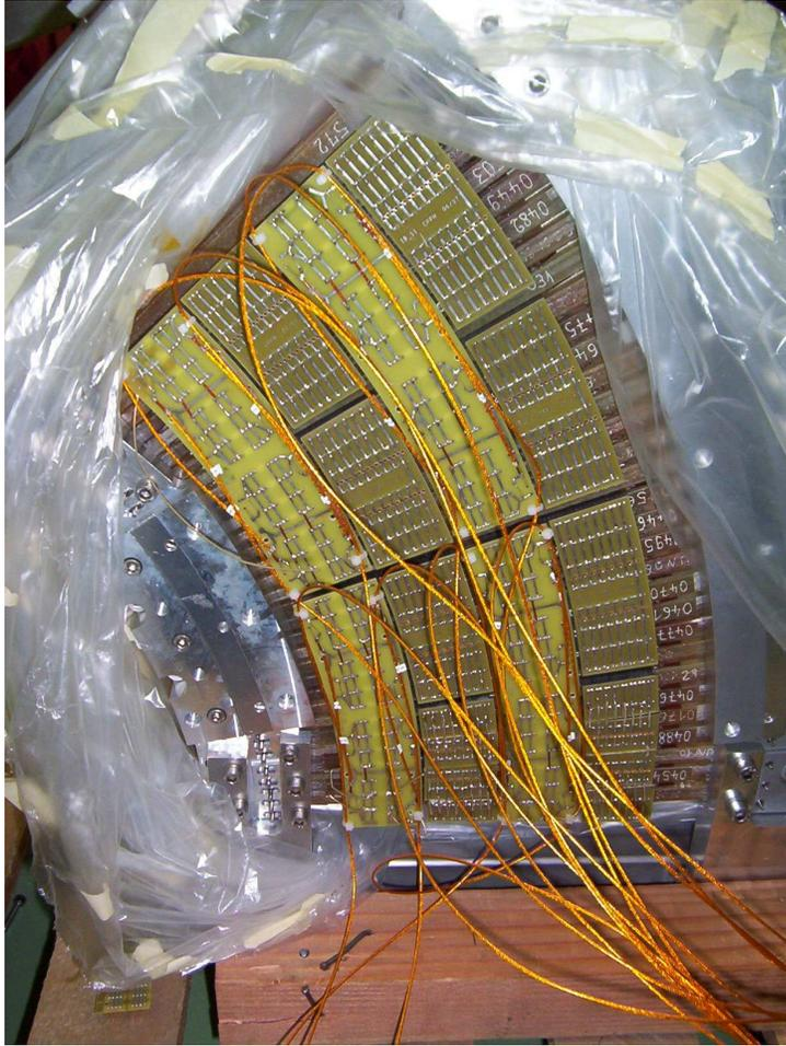
Figure 4.2: Photos of EMEC summing board.
