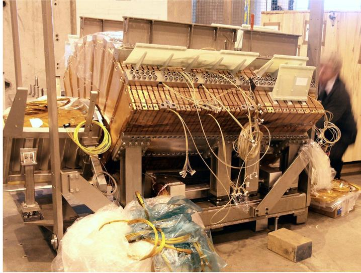
Figure 2.20: View of the EMEC module (the small one) and the HEC module.
