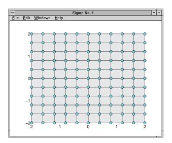
Note that the surface function does not use a 3-D view like the high-level surf functions. Object creation functions simply add new objects to the current axes without changing axes properties, except the Children property, which now includes the new object and the axis limits (XLim, YLim, and ZLim), if necessary.
