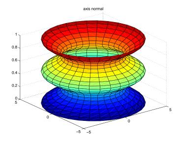
axis square creates an axis that is square regardless of the shape of the figure window. The cylindrical surface is no longer distorted because it is not warped to fit the window. However, the size of one data unit is not equal along all axes (the z-axis spans only one unit while the *x*- and *y*-axes span 10 units each).
