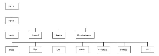
The hierarchical nature of Handle Graphics is based on the interdependencies of the various graphics objects. For example, to draw a line object, MATLAB needs an axes object to orient and provide a frame of reference to the line. The axes, in turn, needs a figure window to display the line.
