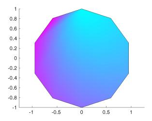
MATLAB now interpolates the colors across the face of the patch. You can color the edges of the patch the same way, by setting the edge colors to be interpolated. The command is:
