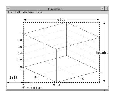
The default 3-D view is azimuth =  $-37.5^{\circ}$ , elevation =  $30^{\circ}$ .
