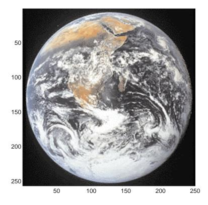
The command axis image works by setting the DataAspectRatio property of the axes object to [1 1 1]. See axis and axes for more information on how to control the appearance of axes objects.
