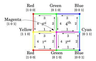
The arrows indicate the order in which each edge is drawn in the first, second, third, and fourth face. The color at each vertex determines the color of the edge that follows it. Notice how the second edge in the first face would be green except that the second face drew its fourth edge from the magenta vertex. You can see similar effects in all shared edges.
