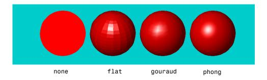
The lighting command (as opposed to the light function) provides a convenient way to set the lighting method.
