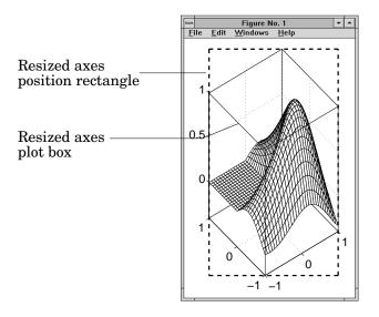
As you can see, reshaping the axes to fit into the figure window can change the aspect ratio of the graph. MATLAB applies stretch-to-fill so the axes fill the position rectangle and in the process may distort the shape. This is generally desirable for graphs of numeric data, but not for displaying objects realistically.
