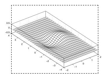
Setting the value of the DataAspectRatio property also sets the DataAspectRatioMode to manual and overrides stretch-to-fill so the specified aspect ratio is achieved.
