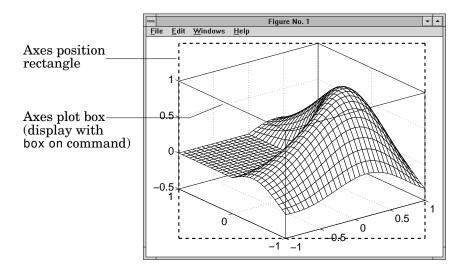
The view is the 2-D projection of the plot box onto the screen.
