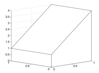
However, this axes distorts the actual shape of the solid object defined by the data. To display it in correct proportions, set the DataAspectRatio.
