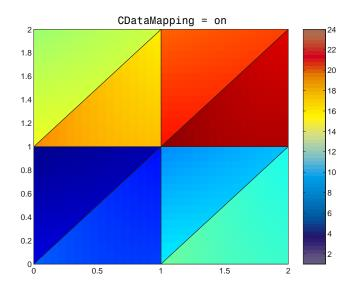
You can alter the mapping of color data to colormap entry using the caxis command. This command uses a two-element vector [cmin cmax] to specify what data values map to the beginning and end of the colormap, thereby shifting the color mapping.
