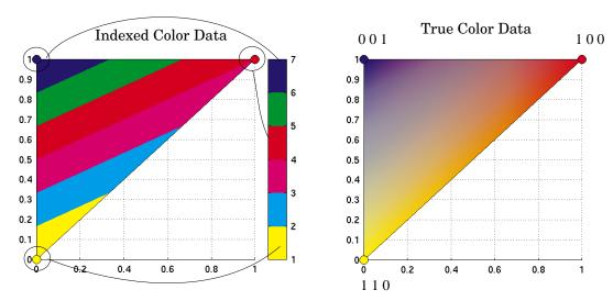
The patch on the left uses indexed colors obtained from the six-element colormap shown next to it. The color data maps the vertex colors to the colormap elements indicated in the picture. With this colormap, interpolating from the cyan vertex to the blue vertex can include only the colors green, red, yellow, and magenta, hence the banding.
