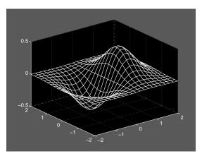
With InvertHardcopy enabled, MATLAB automatically produces output more suited to printing in black and white. Here is the same mesh plot after reversing the color scheme.
