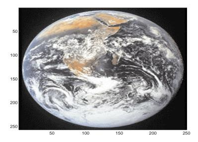
The elongated globe results from stretching the image display to fit the axes position. Use the axis image command to force the aspect ratio to be one-to-one.
