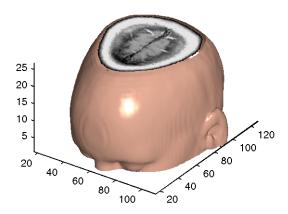
The isocap uses interpolated face coloring, which means the figure colormap determines the coloring of the patch. This example uses the colormap supplied with the data.
