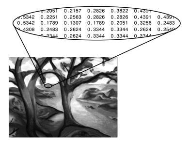
To display an intensity image, use the imagesc ("image scale") function, which enables you to set the range of intensity values. imagesc scales the image data to use the full colormap. Use the two-input form of imagesc to display an intensity image. For example,
