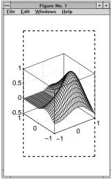
Setting the CameraViewAngle property disables stretch-to-fill, and also prevents MATLAB from readjusting the size of the axes if you change the view.
