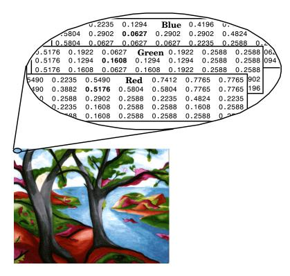
To determine the color of the pixel at (2,3), you would look at the RGB triplet stored in (2,3,1:3). Suppose (2,3,1) contains the value 0.5176, (2,3,2) contains 0.1608, and (2,3,3) contains 0.0627. The color for the pixel at (2,3) is:
