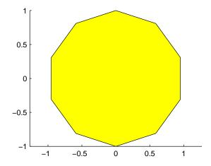
The first and last vertices need not coincide; MATLAB automatically closes each polygonal face of the patch. In fact, it is generally better to define each vertex only once, particularly if you are using interpolated face coloring.
