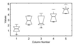
The following example comes from a study of material strength in structural beams Hogg (1987). The vector, strength, measures the deflection of a beam in thousandths of an inch under 3,000 pounds of force. Stronger beams deflect less. The civil engineer performing the study wanted to determine whether the strength of steel beams was equal to the strength of two more expensive alloys. Steel is coded 1 in the vector, alloy. The other materials are coded 2 and 3.
