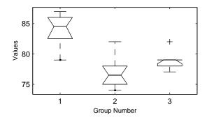
The p-value indicates that the three alloys are significantly different. The box plot confirms this graphically and shows that the steel beams deflect more than the more expensive alloys.
