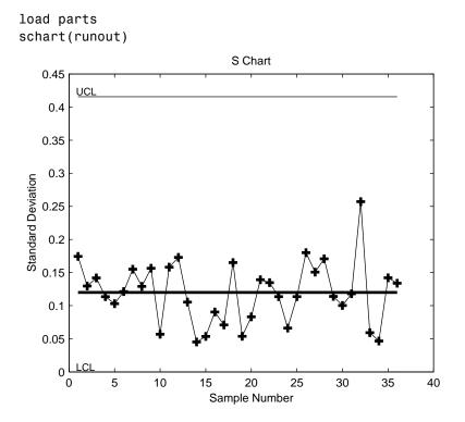
in thousandths of an inch, the amount the part radius differs from the target radius.
