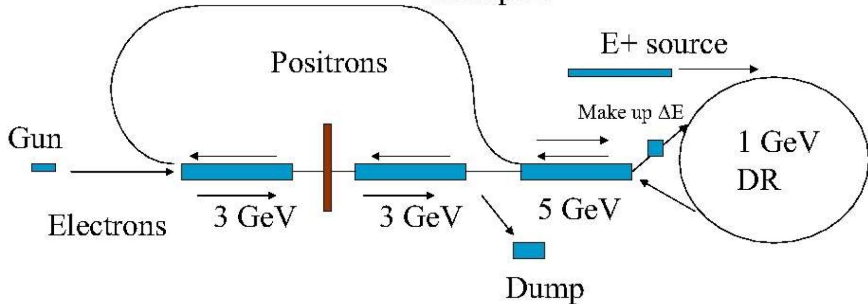
A small version of the ILC that runs at the  $\Upsilon(4s)$ , with a reduced boost ( $bg \sim 0.1-0.2$ ) and a better vertex resolution (thanks to smaller beam-spot and limited multiple scattering).
